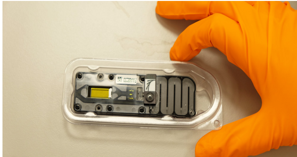
A Nanopore flow cell for the MinION. | Photo from Science Practice http://www.science-practice.com/blog/2016/04/22/minion-burn-in/
